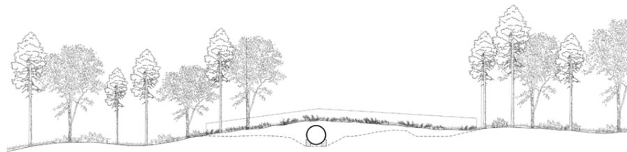
Section of the ecological passage with existing and new terrain
